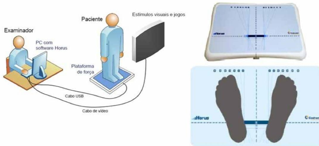
**Figure 1.** Schematic illustration of the functional diagram and positioning of the feet on the platform
